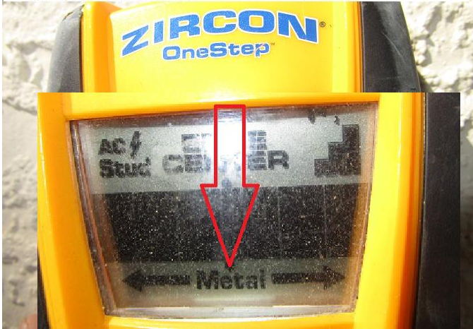
**wall type construction: 100% reinforced masonry
