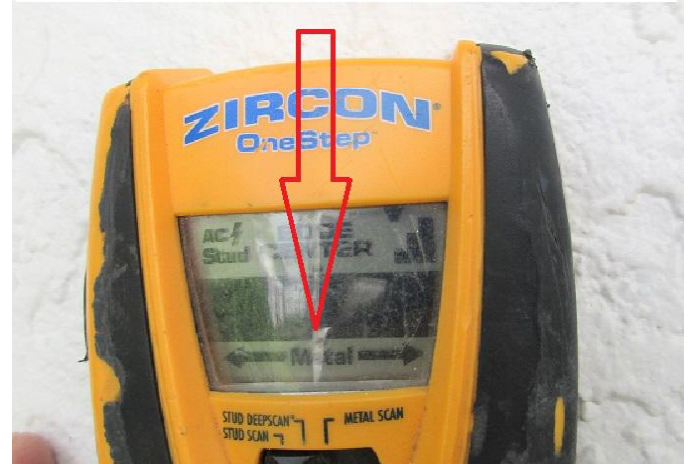
**wall type construction: 90% reinforced masonry
