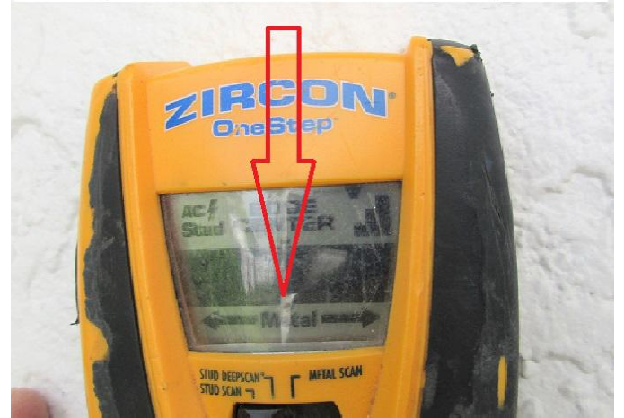
**wall type construction: 90% reinforced masonry
